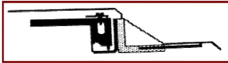
The edge sensor is used to mechanically sense when the probes have touched and after overdrive has been applied. When the switch contact opens it signals the tester to begin the test sequence. To prevent contact arcing and oxidation it is important to insure contact BEFORE power is applied to the device. Two edge sensors can be wired in parallel to provide redundancy in the event of failure of one of the switch contacts.
